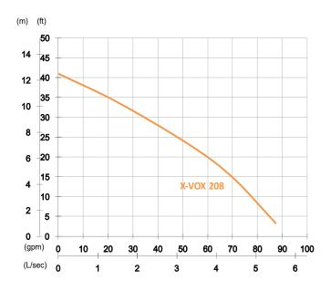
Shaft Speed: 3450 rpm Outlet: 50mm, 2in
